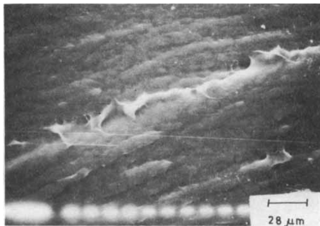
FIGURE 15 Tensile failure surface of H 50 showing ductile failure with a central stress path.
